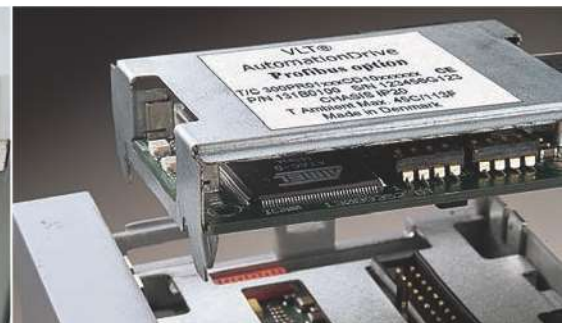
The fieldbus option plugs in beneath the front panel. It can be turned upside down to allow for cable entry on top.
